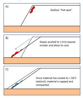
Figure 5 Spontaneous combustion remediation option 1 (R1) for shallow affected materials.
