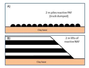
Figure 6 Spontaneous combustion Emplacement Facility.
