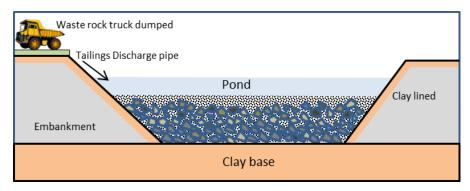
Figure 3 Co-disposal of tailings and waste rock (including reactive PAF).
