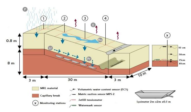
**Figure 1** 3D schematic representation of the field instrumented cell (E: evaporation; P: precipitation; R0: runoff; Pr : percolation; Lf: lateral flow); locations 1 to 4 on the slope are the monitoring stations
