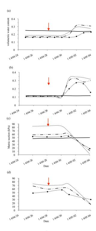
**Figure 4** Measured volumetric water content at depths of 75 cm (a) and 50 cm (b) and measured matric suction at the depth of 75 cm with Watermark (c) and Jetfill (d) stations (the arrow in the figure indicates the wetting event)
