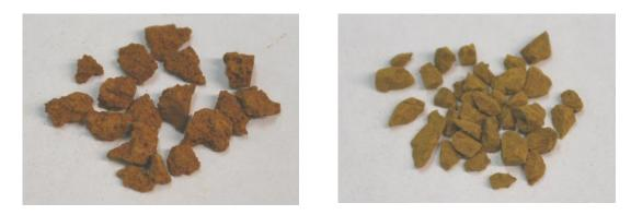
**Figure 3** SHM-based adsorbents, obtained by mixing with an organic polymer (left) and high pressure compaction, crushing and sieving (right). Grain size: 1-2 mm in both pictures
