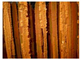
**Figure 1** 1-2.5 m<sup>3</sup>/h pilot plant in Tzschelln (left), where schwertmannite is generated as a byproduct of microbial catalysed lignite mine water treatment on special carrier elements (right)
