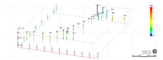
**Figure 7** 3D schematic diagram of the OTD showing sample locations and sulphide alteration index (SAI) values. Zones A to D are indicated (by thick black lines) and the northern pond is shown in Zone D.
