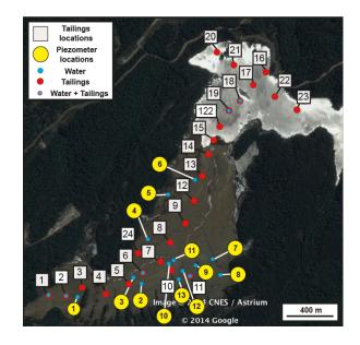
**Figure 2** Plan view map of the Old Tailings Dam showing tailings sample locations (red; n=24), and water collection locations (blue). Established piezometer locations are shown in yellow circles (image from Google).
