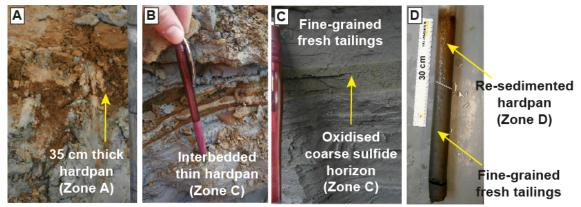
**Figure 3** Examples of tailings oxidation observed in the OTD. A: Thick oxidised hardpan (30 to 35 cm depth) prevalent in Zone A; B: Thin hardpan layers interbedded within fresh tailings packages at depth (c.1 m; Zones B and C); C: Coarse oxidised sulphide horizon observed in Zones B and C; D: Re-sedimented hardpan seen in Zone D.
