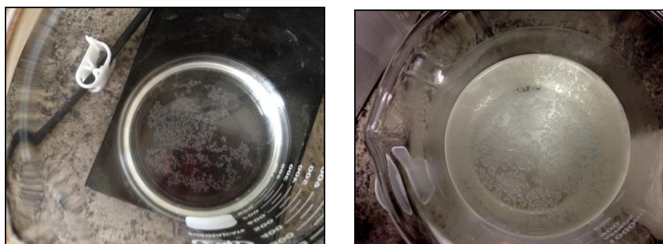
Figure 5 A) Precipitate that formed from the deep pit water control over a period of 3 days. B) Groups of precipitated crystals that occurred at the surface during heating of the deep pit water.
