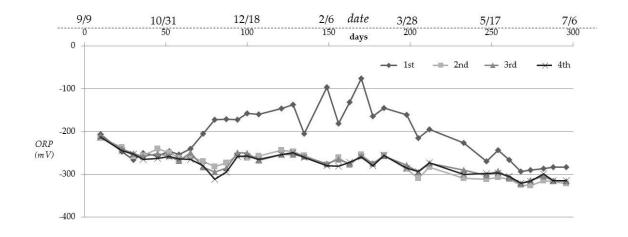
Figure 5 Changes in the ORP values over time in the anaerobic bioreactor.
