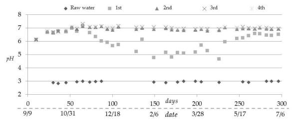
Figure 4 Changes in the pH values over time in the anaerobic bioreactor."1st, 2nd, 3rd, and 4th denote the location at which the sample was drawn"
