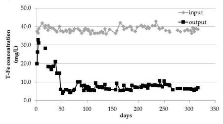
Figure 2 Changes in the concentrations of T-Fe in the mine drainage before and after treatment in the ironoxidation removal bioreactor.
