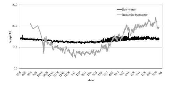
Figure 3 Changes in temperatures of raw mine water and inside the anaerobic bioreactor throughout the year.
