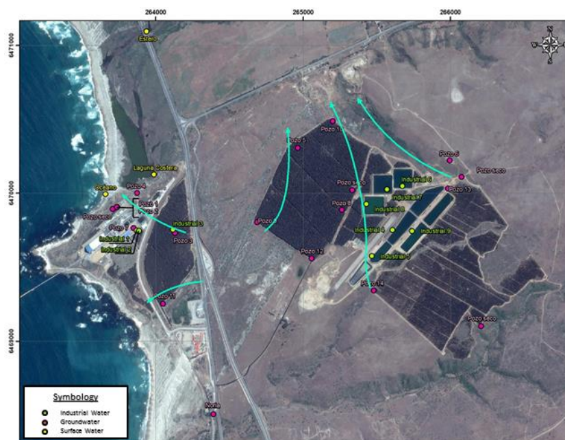
Figure 4 Sampling points and groundwater flow directions in the Pilot Basin where Sulfate is the main concern in the groundwater (coastal area).
