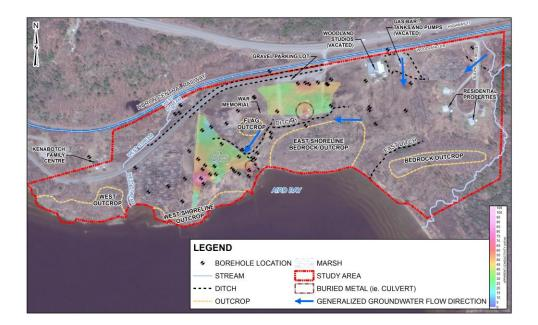
Figure 4 Electromagnetic geophysical survey results (mS/m)
