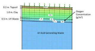
Figure 7 BRSF cover oxygen penetration
