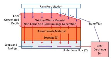
Figure 8 BRSF geochemical conceptual model
