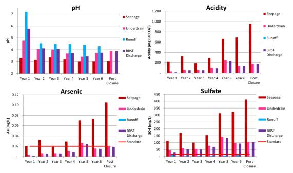
Figure 9 BRSF discharge water quality predictions
