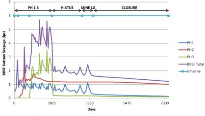
Figure 6 Predicted BRSF seepage flows vs. time
