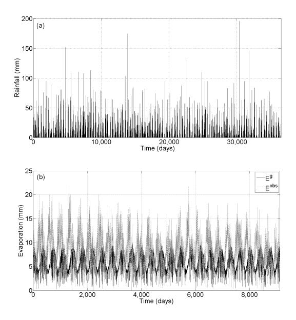
**Figure 2** Examples of generated time-series of daily (a) rainfall and (b) evaporation values based on historical weather observations in Mount Isa. The generated evaporation values E<sup>g</sup> underestimated the observed evaporation values E<sup>obs</sup>.
