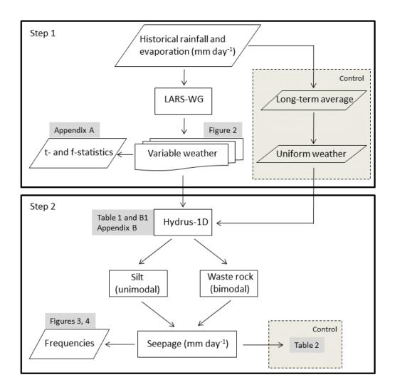
**Figure 1** Schematic diagram of a climate-based planning framework for cover systems. Step 1 generates time series of rainfall and evaporation based on historical observations. Step 2 uses the generated weather data to assess frequency distributions of seepage based on selected soil materials. In total, we generated 35 time-series, each of 100 years length.
