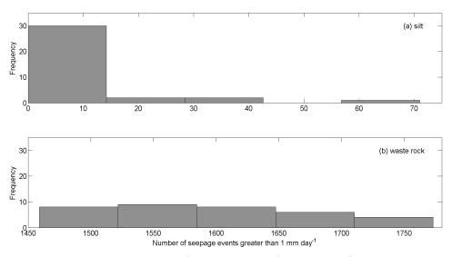
**Figure 5** Frequencies of number of events with seepage greater than 1 mm day<sup>-1</sup> for (a) unimodal silt and (b) bimodal waste rock material and variable climatic conditions (based on 35 generated time-series, each of 100 years length). Note the scale differences.
