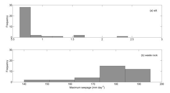
**Figure 4** Frequencies of maximum seepage for (a) unimodal silt and (b) bimodal waste rock material and variable climatic conditions (based on 35 generated time-series, each of 100 years length). Note the scale differences.
