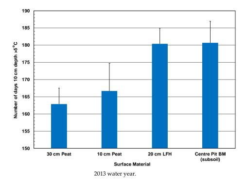
Figure 5 Number of days soil temperature at 10 cm depth was greater than 5°C for surface materials during the 2012 - 2013 water year.
