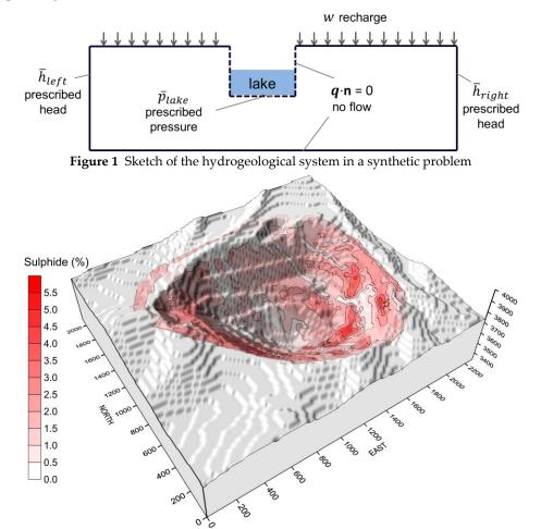
Figure 2 Sulphide distribution in the wall of a final open pit
