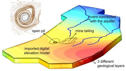
Figure 6 Hydraulic head distribution
