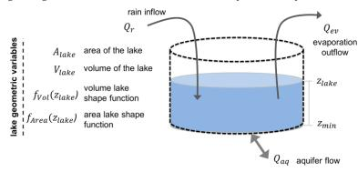
Figure 3 Sketch of the lake system in a synthetic problem
