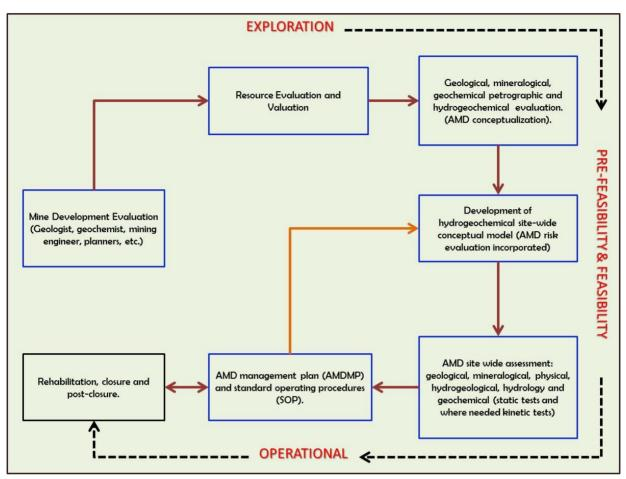
Figure 3 Flow Diagram to be adopted at the Exploration Stage
