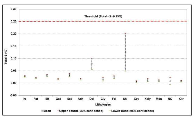
Figure 2 95% Confidence Intervals for Waste Lithologies at Deposit C
