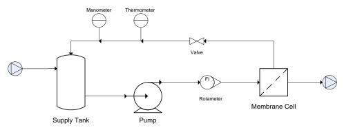
Figure 1 Schematic of NF unit
