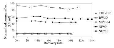
Figure 3 Normalized permeate fluxes of the five membranes as a function of effluent recovery rate
