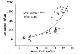
Fig. 4 The relationship between gas output and water yield by well B07
