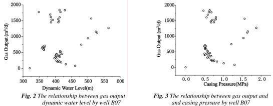
Through the representative well of limited information, gas output process can be seen: by maintaining the dynamic water level reasonably, casing pressure is controlled with reason relatively, great help can be made for gas output increasing of CBM wells.
