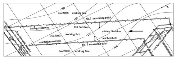
Fig. 3 Schematic plane diagram of measurement borehole in roadway on 21021working face
