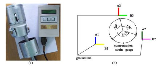
(a) Photos of sensor and strain recorder **Fig. 2** The sketch of borehole measuring device
