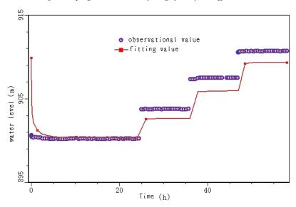
Fig.4 Pumping test water table fitting of 2# hydrology borehole
