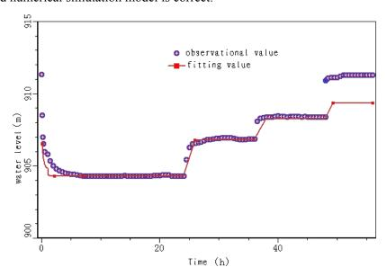
Fig.3 Pumping test water table fitting of 1# hydrology borehole
