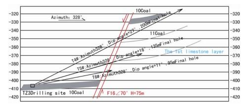
Fig.2 Searching profile of F16 fault
