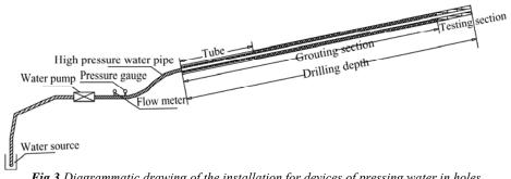
Fig.3 Diagrammatic drawing of the installation for devices of pressing water in holes
