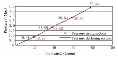
Fig.4 Curve chart of flow rate and pressure for high pressure pressure water test
