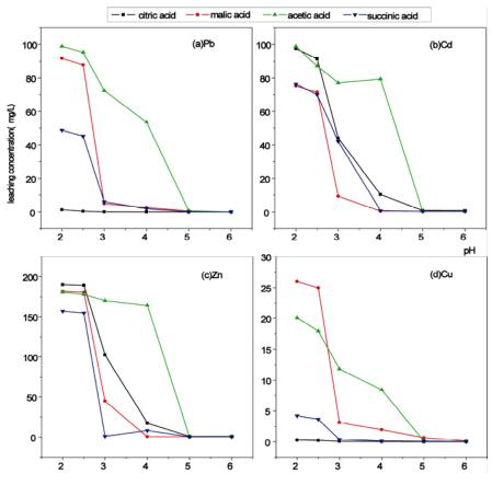
Fig.2 Effects of different organic acids and pH on the heavy metals leaching
