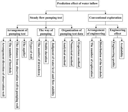
Fig. 1 Evaluation index system of wellbore water inflow prediction effect.
