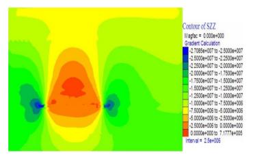
Fig. 5 stress cloud chart of surrounding rock at 140 m in working face
