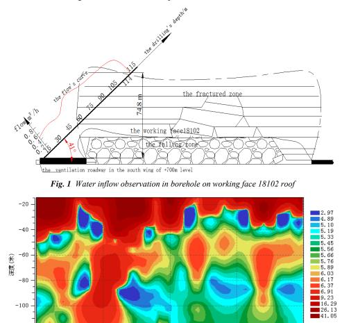
Fig. 2 Apparent resistivity chromatogram along Inclined 60 degrees
