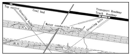
Fig. 3 Diagrammatic profile of grouting reconstruction
