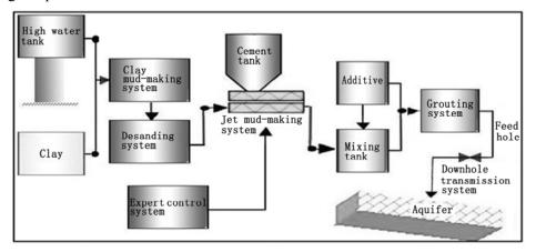
Fig. 4 Process flow chart of grouting reconstruction
