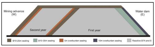
Fig. 3 Second year compartment of inter-burden benches 7A and 8.(Redrawn from Adamski 2003.)
