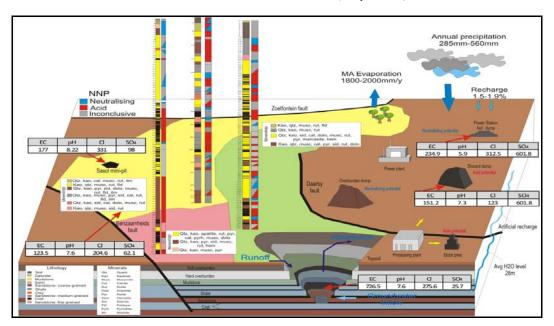
Fig. 2 Summary of the acid and neutralising potential of the various contributing factors over the extent of the study area.
