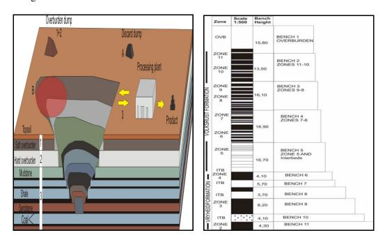
Fig. 1 Open cast mining in the study area illustrating the waste generated at various phases during mining (Left); Stratigraphic column with the lithological units and benches mined in the Waterberg Coalfield (Right).
