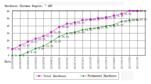
Fig. 4 Water hardness change curve of the water inrush points in Roadway II51
