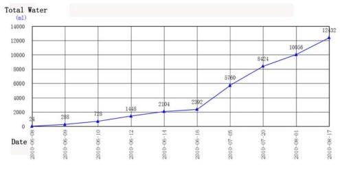
Fig. 2 Aggregate flow curve of the water point 28.5m ahead of Roadway II5<sub>1</sub>(-720 m)
