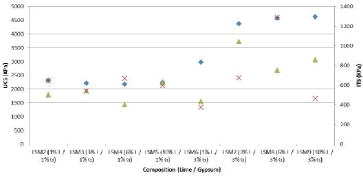
◆ UCS (4hrs curing)(KPa) ▲ UCS (7days curing) (KPa) ×ITS (KPa)
