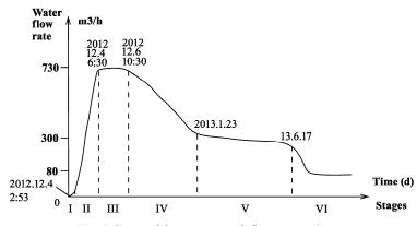
Fig. 2 Curve of the water inrush flow rate with time I - water gathering stage; II - rapidly increasing water stage; III - constant maximum flow rate stage; IV - declining water flow rate stage; V - flow rate stabilizing stage; VI – second water declining and stabilizing again stage
