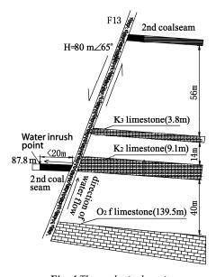
*Fig. 4 The geological section map near the water inrush point.*
