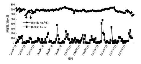
Fig. 3 Relation of atmospheric water and No. 8 mine inrush
