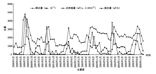
Fig. 2 Relation of atmospheric water, Zhan-river recharge and No.7 mine inrush
