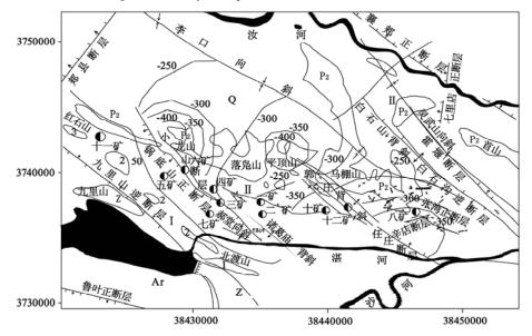
Fig. 4 Isoline map of Cambrian karst groundwater level in mine area
