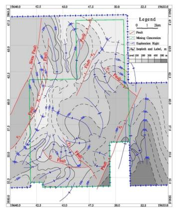
Fig. 2 Areal structure of No.3 Coal Bed in Fanzhuang Block
