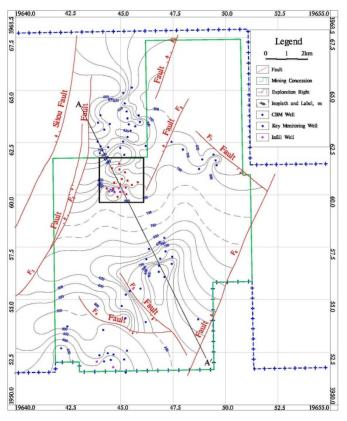
Fig. 3 Groundwater fluid potential in Fanzhuang Block
