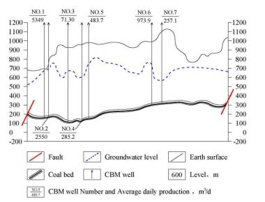
Fig. 6 Groundwater fluid potential and daily gas productions of CBM wells in Profile AA'
