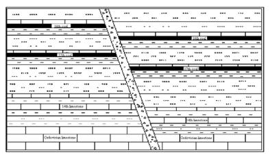
Fig. 2 The sketch map of prototype fault in model test
