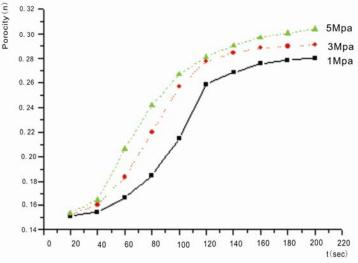
Fig. 11 n -curve of No.1 fault water inrush under different pressure
