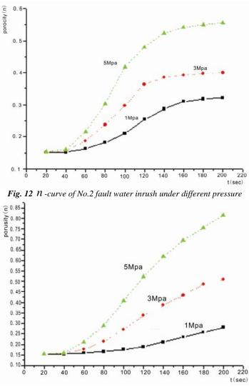
Fig. 13 *N*-curve of No.3 fault water inrush under different pressure
