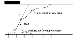
Fig. 4 The sketch of Mining fault water-inrush
