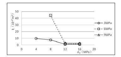
Fig. 4 Permeability confining pressure effect
