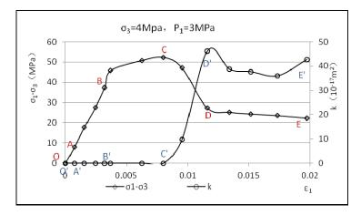
Fig. 3 Whole stress strain permeability curves
