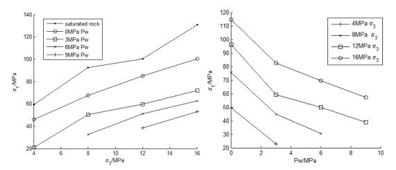
Fig. 1 Fine sandstone strength confining pressure effect Fig. 2 Fine sandstone strength pore pressure effect
