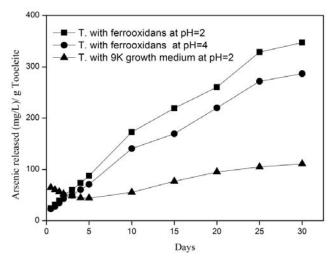
Fig. 4 Arsenic released from tooeleite with time under ferrooxidans culture and medium at pH=2 and 4
