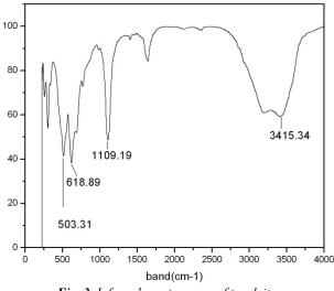
Fig. 3 Infrared spectroscopy of tooeleite
