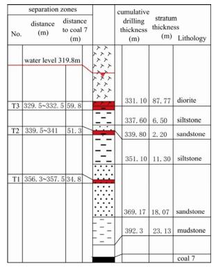
Fig. 3 The position of separation zones by flow rate logging results in borehole R455
