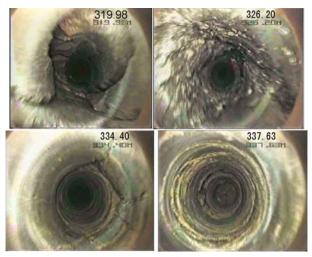
Fig. 2 The borehole TV picture of separation zones in siltstone and medium sandstone
