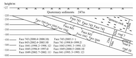
Fig. 1 Inclination profile of working face 745
