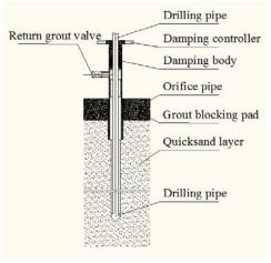
Fig. 2 grout protected orifice device schematic
