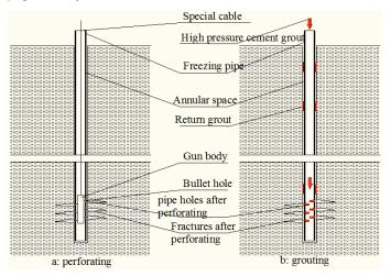
Fig. 4 Perforating grouting principle schematic
