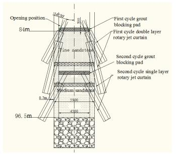
*Fig. 3 Double cycle rotary jet grouting curtain schematic*
