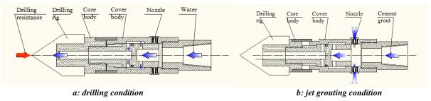
Fig. 1 Drilling-jetting integrated tool schematic
