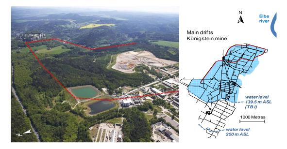
Fig. 1 Left: View of the Königstein mine site/Germany (Background: Elbe river and National Park); Right: schematic map of main drifts with flooded sector (blue) and control drifts (red)
