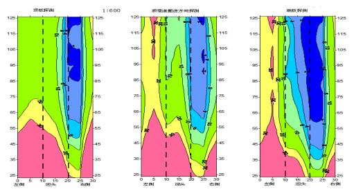
Fig.3 Apparent resistivity abnormal areas in the working face of roadway 720
