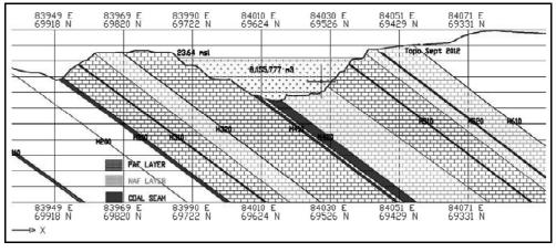
Fig. 2 Typical cross-section of M4E pit geology
