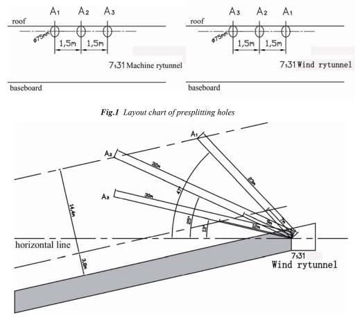
Fig. 2 Designed layout chart of presplitting holes
