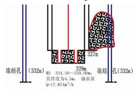
Fig. 1 Layout diagram of the grouting pad and lodgement at the bottom hole
