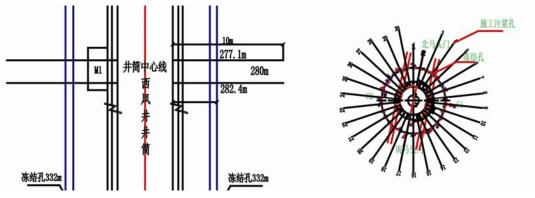
Fig. 2 Layout diagram of M1 aquifer and the annulus outside the freezing pipe wall
