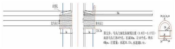
Fig. 5 Layout diagram of advanced exploration and preliminary grouting holes of ingate
