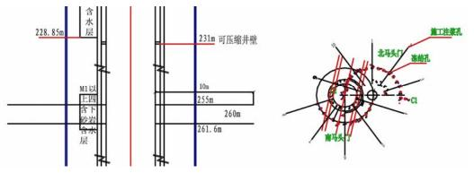
Fig. 3 Layout diagram of grouting holes in the sandstone formation between M1 and the "fourth aquifer"
