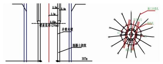
Fig. 4 Layout diagram of grouting holes in the upper section (307m) of ingate
