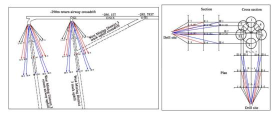
Fig. 1 Layout plan of drill holes for advanced curtain grouting
