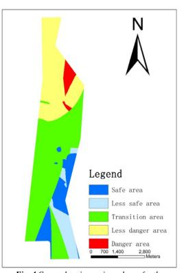
Fig. 4 Comprehensive zoning scheme for the water-inrush risk assessment of the No. 8 coal seam roof
