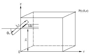
Fig. 3 Location infinite space aquifer inclined line sink and observation points
