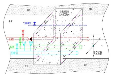
Fig. 2 Structural Diagram of Waterproof Sealing Wall
