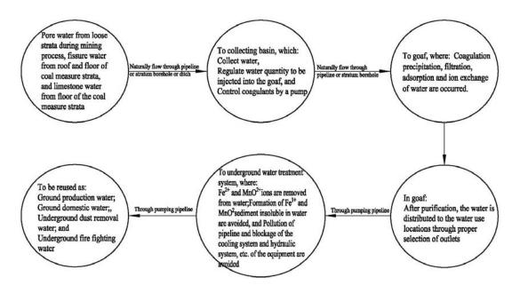
Fig. 1 Process flow diagram for mine water reuse in underground goaf
