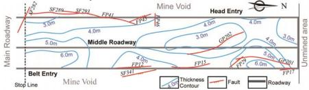
*Fig. 1 Plan view map of 163L02C coal mine panel. Map plots the layout of roadways, the contours of coal bed thickness and true fault traces (fault throw*  $\leq 1.5$  *m).*
