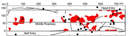
Fig. 2 Stress-concentration zones (red color) and high-energy microseisms (black point) in 163L02C panel. Black lines are true fault traces as fig.1 shown.
