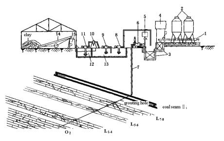
Fig. 1 The diagram of the floor consolidation grouting system 1-screw conbeyor; 2-bulk cement tank;3-mixer;4-overhead water-tank;5-additive tank;6-grouting pump;7grouting pipe;8-slurry pump;9-circulating pump;10-cyclone;11-vortex pump;12-pulp pool;13-seminal plasma pool;14-belt converyor;15-pulping machine
