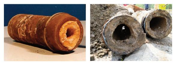
Fig. 1 Boring pipe from coal mine (a: left) and of the pipeline of the Olza Collector (b: right)
