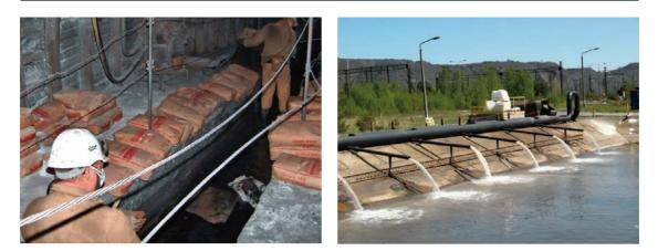
Fig. 2 Feedres of sodium sulphate: in mine working (left) and on the surface (right)
