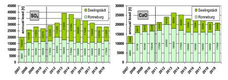
Figure 2 Measured and predicted released loads of sulphate and hardness (as CaO) based on the planned remediation progress
