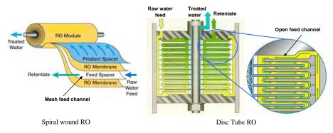
Figure 3 RO module configurations
