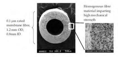
Figure 2 PVDF Hollow fibre filtration membrane
