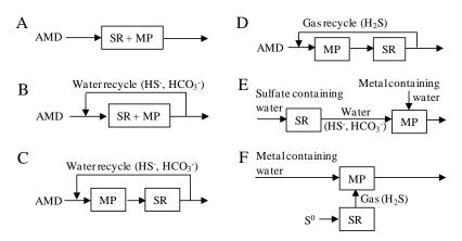
**Figure 2** Possible configurations of bioreactor processes for acid mine drainage (AMD) treatment and metal recovery. SR = sulfate or sulfur reduction, MP = metal precipitation (adapted from Hao 2000; Kaksonen and Puhakka 2007).
