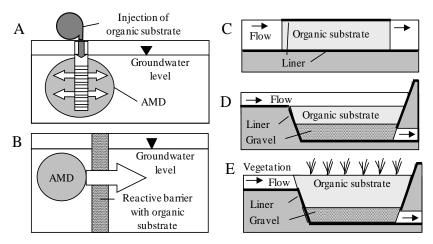
**Figure 1** Passive, sulfate reduction based applications for treatment of acid mine drainage (AMD): (A) injection of substrates into the subsurface, (B) permeable reactive barriers, (C) infiltration beds, (D) anoxic ponds, (E) anaerobic wetlands, adapted from (adapted from Kaksonen and Puhakka 2007).
