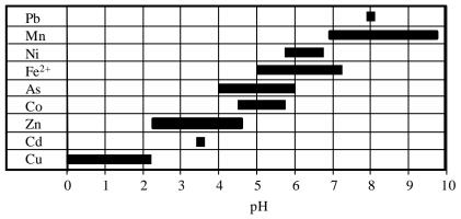
Figure 3 Used and/or recommended pH values for the selective precipitation of metals as sulfides (adapted from Hammack et al. 1994; Govind et al. 1997; Tabak et al. 2003; Kaksonen and Puhakka 2007)
