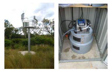
Figure 3: Receiving waterway station (Left: elevated platform. Right: automatic sample
