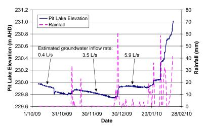
Figure 9: Groundwater inflow estimation for pit
