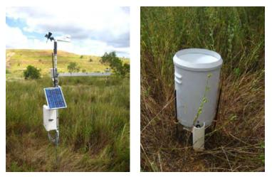
*Figure 2:* Mine weather station (Left: main station. Right: tipping bucket rain gauge)
